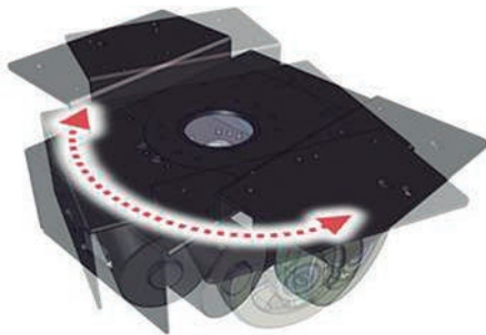
▲ 차동 구동 ( DD : Differential Drive )
