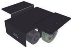
차동구동 ( DD : Differential drive )
